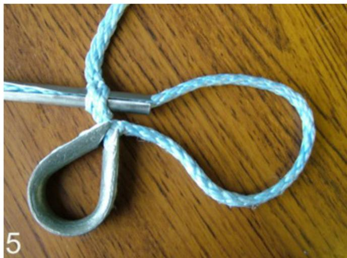
You should now insert the fid as in picture 4 of the long splice, i.e. skip two holes and enter the third, and with the fid at approximately 45 degrees to the standing part, exit at the fourth hole along. You end up with this picture 5 matching the state of play in picture 5 of the long splice.
