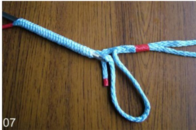
To complete the splice, you need to bury the working end completely inside the tubular braid of which the rope is made. To do this take the darning needle and open up the strands as you did with the fid, but instead of coming out of the other side of the rope, you push it up inside the rope.
