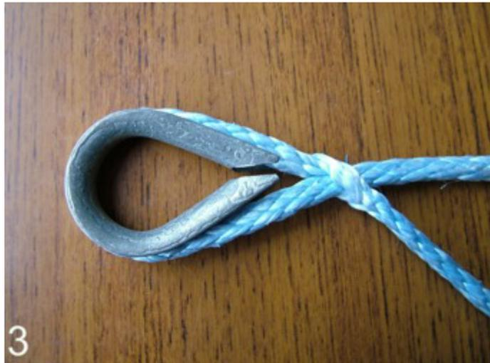
The remaining kink can now be smoothed out, by pulling the working end, and its continuation in the eye. Smooth the kink out, with your fingers, until it looks like a normal splicing hole. You will now have a simple eye with a normal looking standing part and working part.
