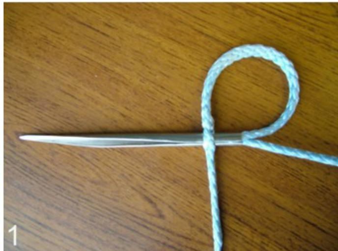
The eye splice is started in a different way to the long splice, but the finishing off is identical.
