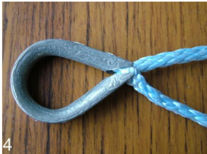
This picture shows the standing part at the top, and the working part at the bottom. The benefit of this technique of creating an eye, is that it will tend to tighten under load, but the conventional method of inserting a working part into the standing part will tend to undo under load.
