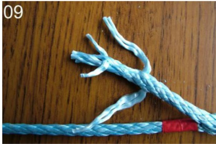
Remove the tape from the working end. Now taper the working end over a distance of a couple of inches, (5cm) by pulling out strands at differing lengths,
